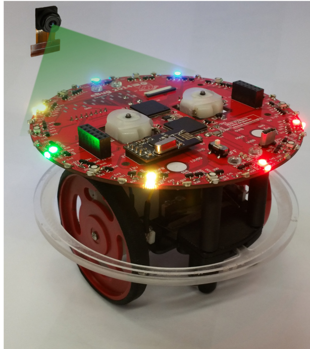
Fig. 1. An eBug displaying a colour sequence on eight of its sixteen LEDs. The camera viewing the eBug can only see three of these LEDs.
